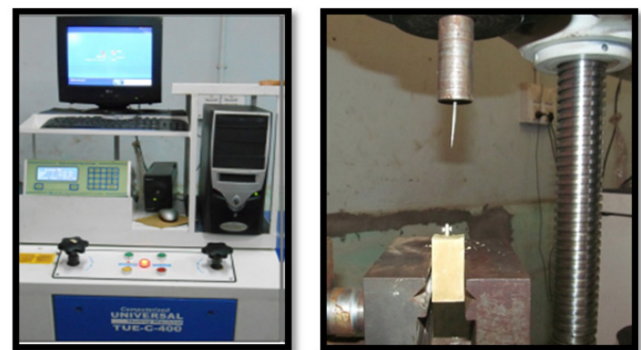
Figure 2: Universal testing machine and customized jig with specimen. (a) Universal testing Machine (b) Customized Jig with specimen.
