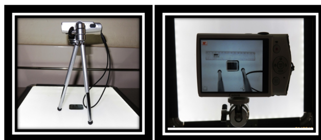
Figure 2: Digitizing the radiograph
